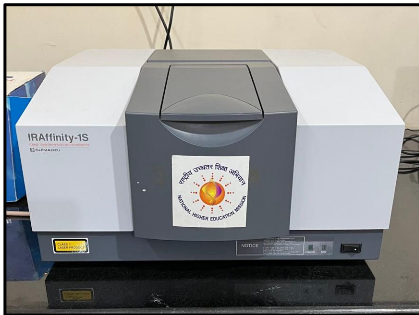
Fourier Transform Infrared Spectrophotometer – IRAffinity – 1S – SHIMADZU
